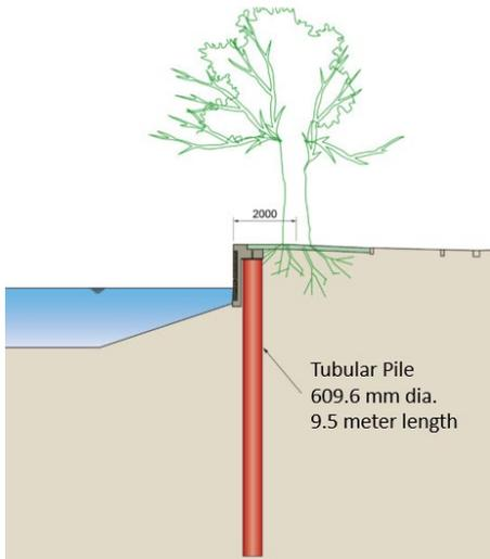
Fig.1 Under construction & Cross section
