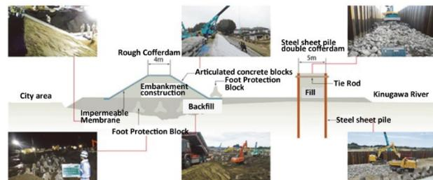
Fig. 2.1 Rough cofferdam, steel sheet pile double cofferdam/standard sectional view<sup>16)</sup> (Provided by Kanto Regional Development Bureau, Ministry of Land, Infrastructure, Transport and Tourism)
