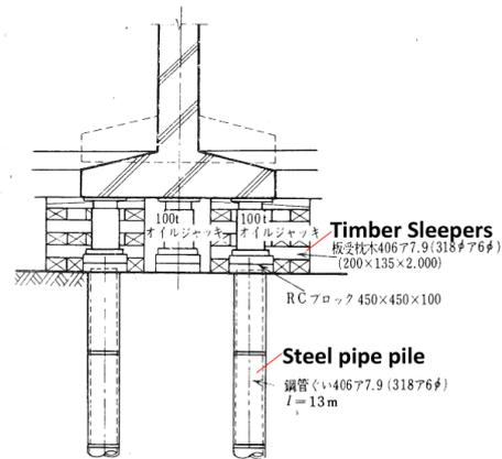
Fig.1.1 Detailed Drawing of Leveling<sup>1)</sup>
