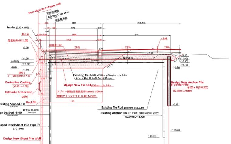
Photo 1.11 New Installation of steel sheet piles of designed water depth - 7m quay<sup>13)</sup>
