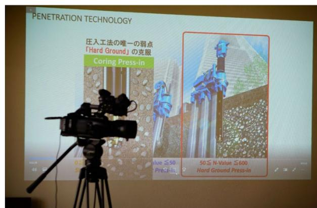
Photo 2. Press-in method to install sheet piles into hard ground
