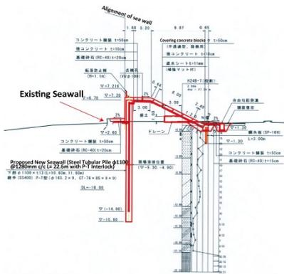
Fig. 1.4 Ishinomaki Port Higashihama coastal seawall standard cross section<sup>14)</sup>
