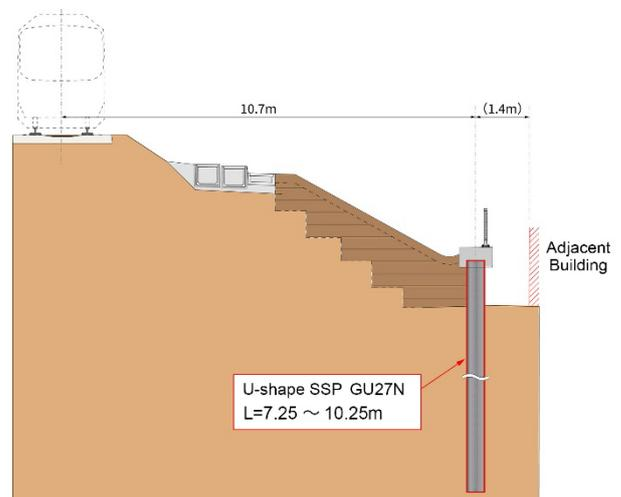
Fig.2 Cross section
